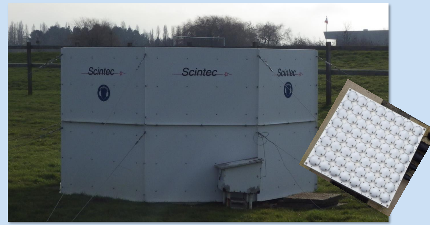
Sodar Sfas Scintec portée 200m Installation 31/07/2014
