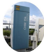
Low power lidar and ceilometer
