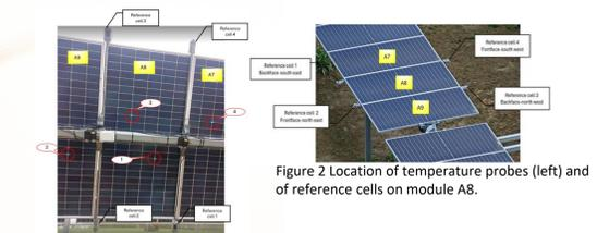
Figure 2 Location of temperature probes (left) and of reference cells on module A8.
