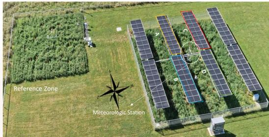
Figure 1 Layout of agrivoltaic installation located on the campus of Ecole Polytechnique in Palaiseau, France.
