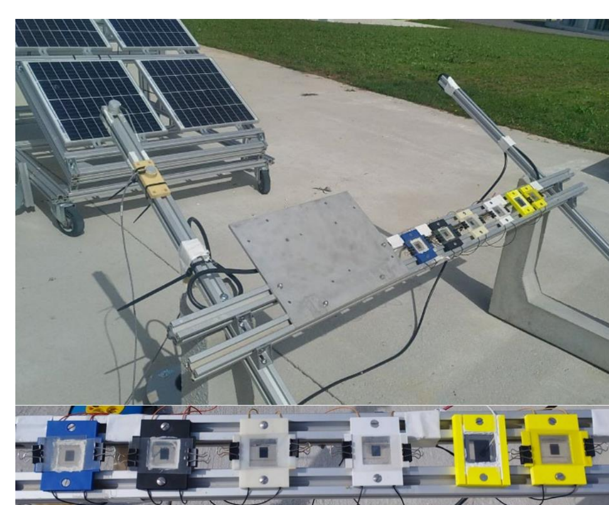
Sirta Atmospheric Research Observatory and perovskite test bench
