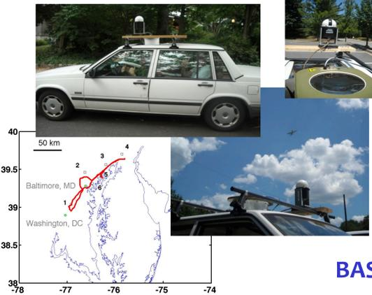
LOA, part of the DRAGON project, equipped a car with a Lidar and photometer (PLASMA).
