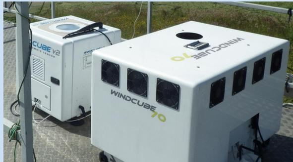
Lidar WLS7v2 Lidar WLS70 Leosphere,
