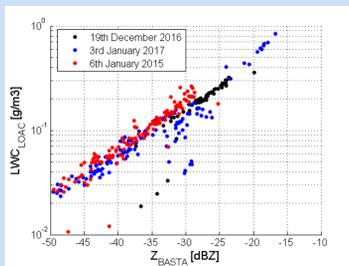
Relationship between Liquid Water Content measured with LOAC sensor and BASTA for the three case studies.
