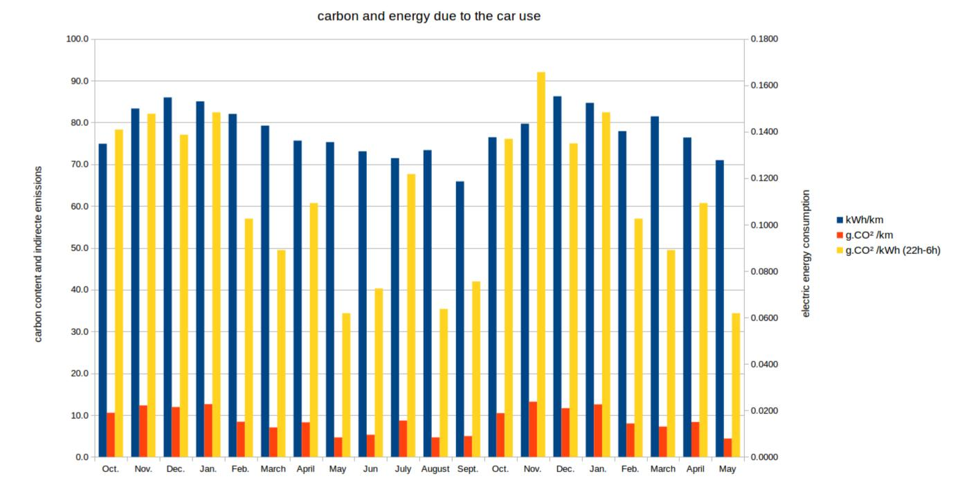
It must be noted that the efficiency is seasonal being lower in winter. This is due to the increased serial resistance in the batteries at low temperature, and to a less extant to the more frequent use of the headlights and the air conditioning. The mean carbon content of the off-peak (22h – 6h) kWh of electricity has been evaluated for each month of year 2017 by sorting randomly 6 days for each month from RTE Data 'Eco2Mix' and making the average.
