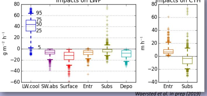
**CONTRIBUTION OF PROCESSES TO CHANGE IN FOG LIQUID WATER BASED ON MEASUREMENTS AND CONCEPTUAL** MODEL (45 CASES).
