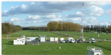
The SIRTA has over 100 instruments on-site, including a profiling mast, ceilometers, particle spectrometers, wind profilers, etc.
