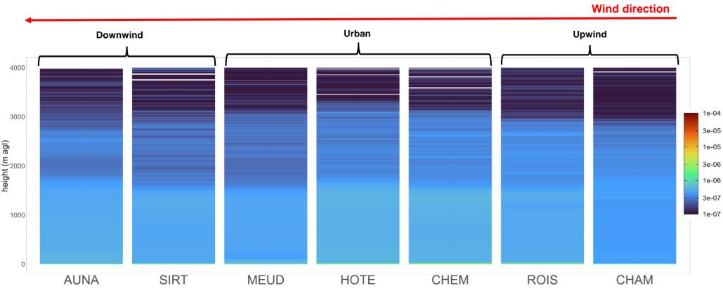
Figure 3. Attenuated backscatter from ALC measurements of the CL61 stations along the dominant wind
