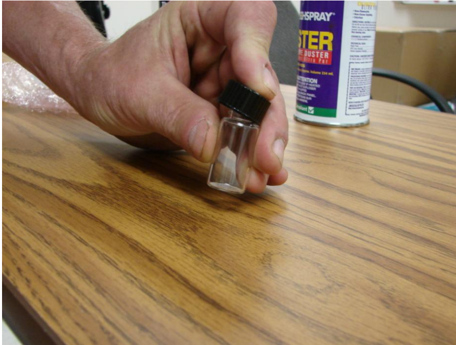
Figure 26: Tapping the Bead Dispenser to Dislodge Beads
