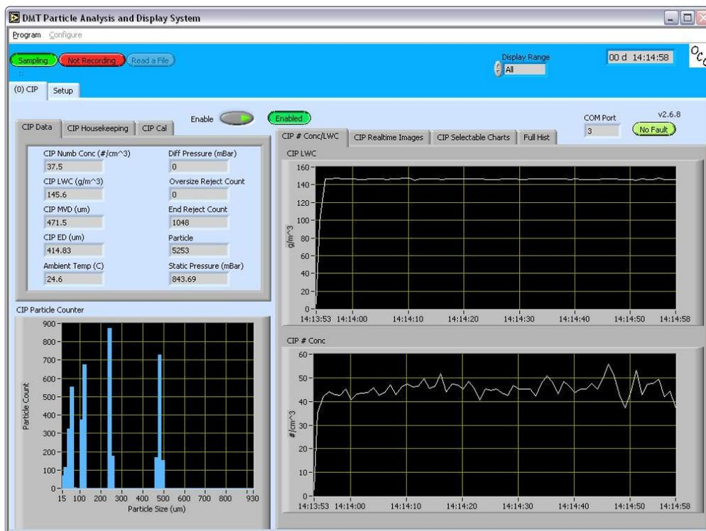
Figure 1: PADS Display Window during Acquisition Mode
